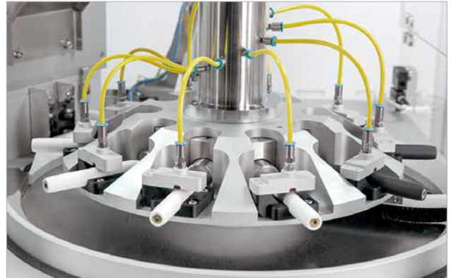
Option: quick-lock holder for HTP products
