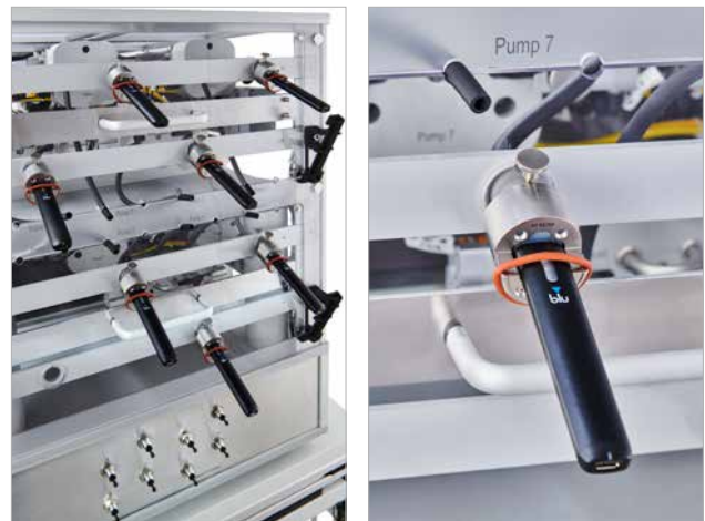
Holder system for ENDS products (e.g. blu)
