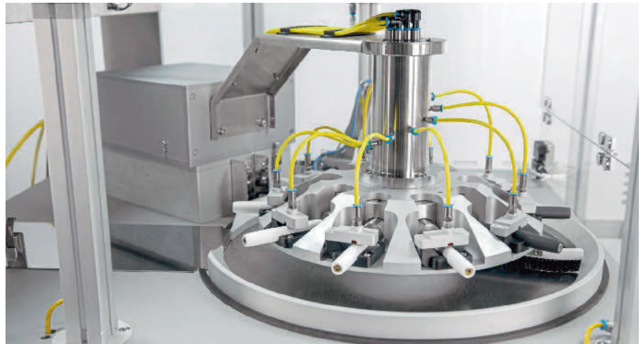
VITROCELL VC 10 S-TYPE: automated and continuous puff generation of Heated Tobacco Products
