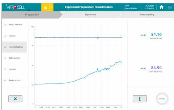
Figure 3: The process wizard indicates the current process step (humidification) and the current progress with target and actual value
