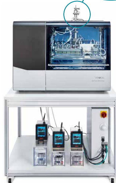
Figure 8: The adaptable PM inlet mounted by small flange quick connector (ISO-KF) on inlet of the AirTox Monitor
