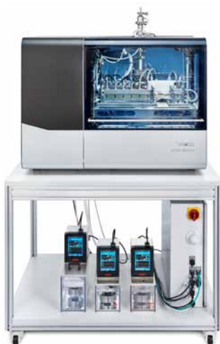
Figure 1: The complete system with AirTox Monitor, control cabinet and water baths.
