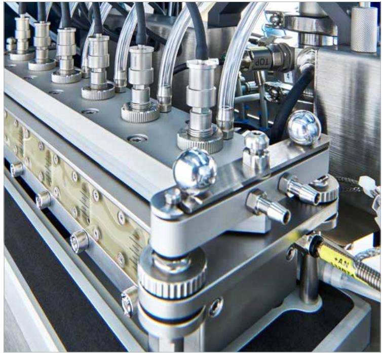
Figure 7: The sample flow is guided to the exposure module, where cell cultures are exposed at the Air/Liquid Interface.
