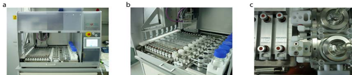
Fig. 1 Semi-automated skin penetration system (SPS) for toxicokinetic studies. a) Complete overview b) Inside view showing the experimental setup with syringes, Franz cells and storage vessels for receptor fluid c) Enlargement of experimental setup showing HPLC vials, receptor fluid in- and outlet and integrated Franz diffusion cells.
